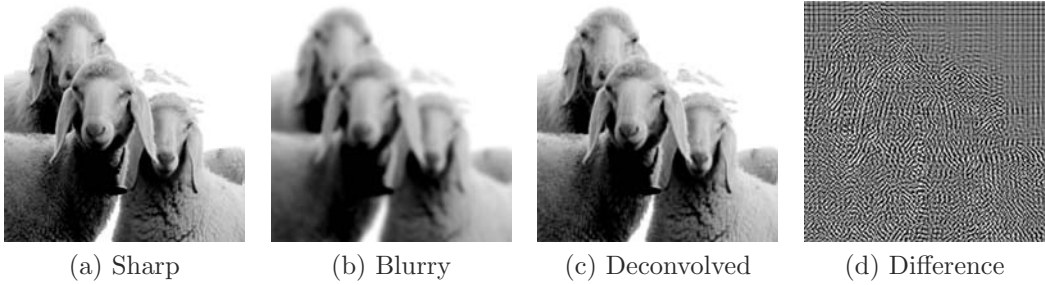
Figure 4.4 Suppose rather than taking (a) the sharp image, we accidentally take (b) a blurry photo; then, deconvolution can be used to recover (c) a sharp approximation of the original image. The difference between (a) and (c) is shown in (d); only high-frequency detail is different between the two images.
