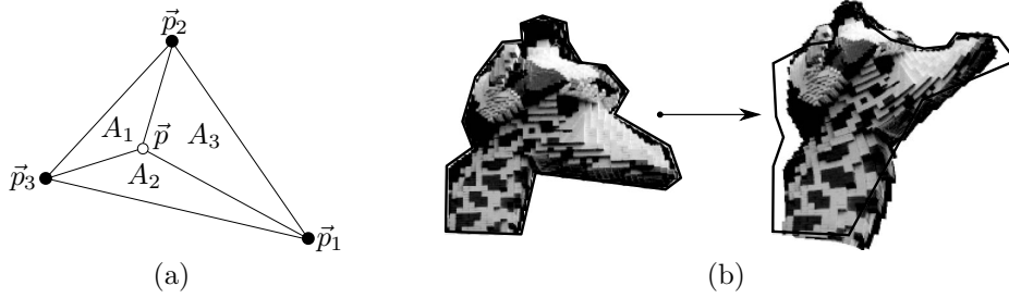
Figure 13.8 (a) The barycentric coordinates of \vec{p} \in \mathbb{R}^2 relative to the points \vec{p}_1 , \vec{p}_2 , and \vec{p}_3 , respectively, are (A_1/A, A_2/A, A_3/A) , where A \equiv A_1 + A_2 + A_3 and A_i is the area of triangle i ; (b) the barycentric deformation method [129] uses a generalized version of barycentric coordinates to deform planar shapes according to motions of a polygon with more than three vertices.
